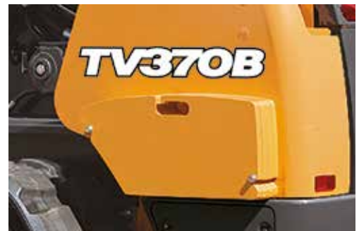
Additional Counterweight to increase ROC
